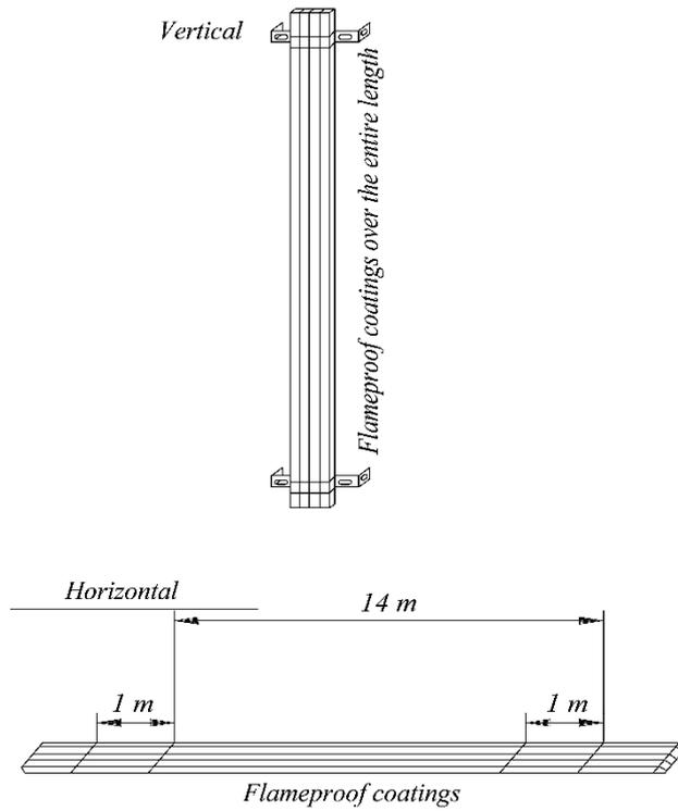
Fig. 16.8.4.3,b. Cable runs protected with flameproof coatings
