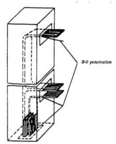
Fig. 16.8.4.3,*a*. Protection of B-0 fully enclosed cable run
