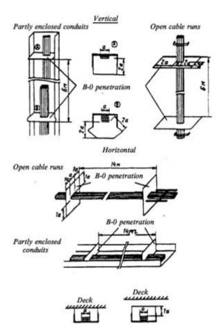
Fig. 16.8.4.3, c. Protection of cable runs with B-0 type fire-retarding structures
