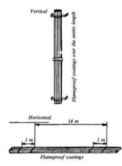
Fig. 16.8.4.3,**b**. Protection of a cable run with flameproof coating
