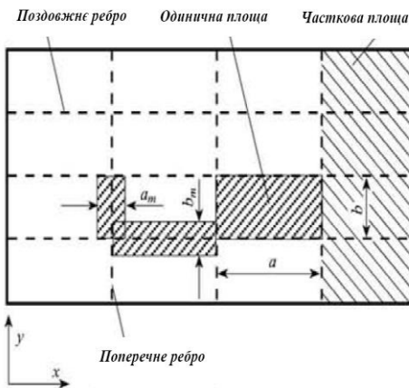
Fig.7.10.6.24 General arrangement of panel
